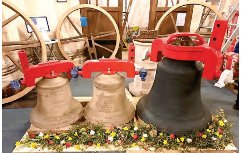
The 500 year-old tenor bell that had its headstock renewed, and the two new bells "Coronation" and "Community", waiting to be hung in the tower. (Photo by Christopher Cadd)
